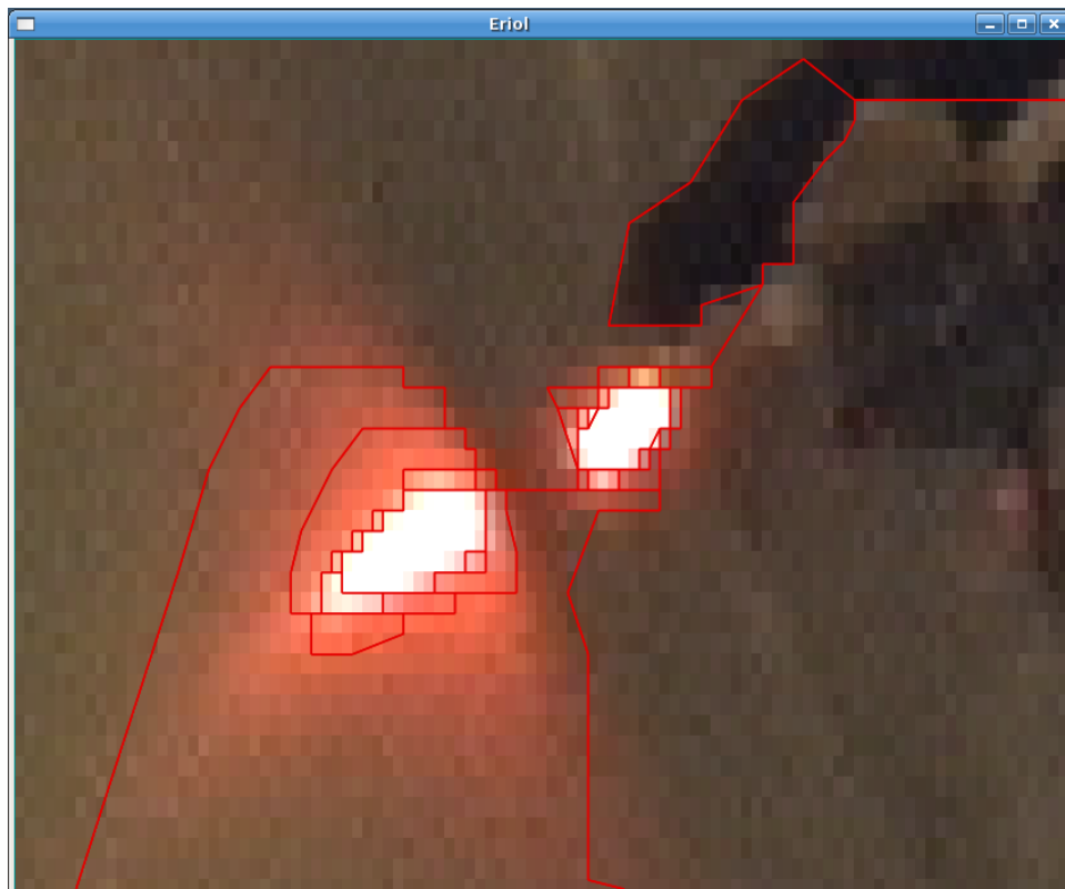
Figure 7: A segmented image in Eriol. The upper-right bright spot is the actual orange LED, whereas the bottom left one is its reflection.
